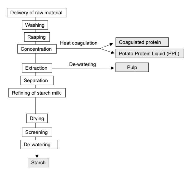
Figure 2: Schematic description of potato starch processing
